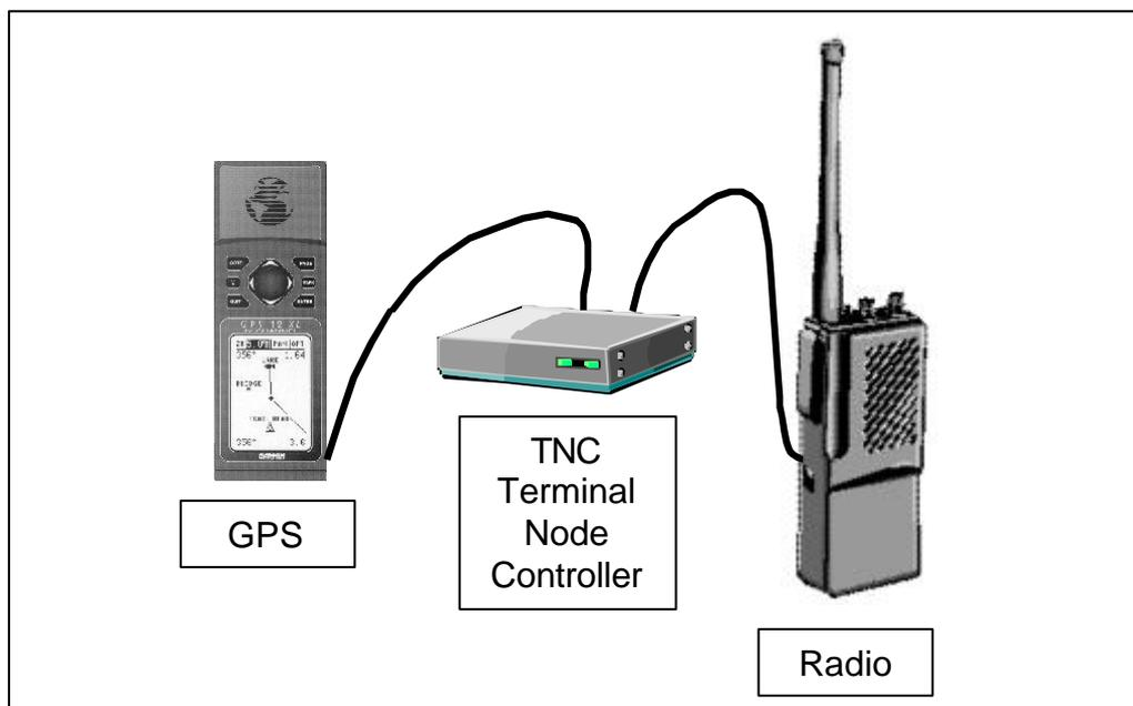
At the control centre, the incoming signal can be decoded by another TNC, and then directed to a serial port on the computer. As each TNC can be programmed separately, each rescue team member can be individually tracked on the map on the computer screen. If required, the progress of each person can be recorded with a trace, or 'snail trail'. The map can be saved and printed as a record of the ground covered. Areas not searched are quickly identified using this technology.
