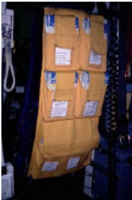
A custom pocket system fastened to the back of the copilots seat provides storage for all the map coverage for the area serviced by this helicopter.
