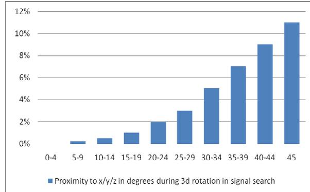
Fig 1b: Loss of range due to suboptimal 3d rotation of the receiving device.
