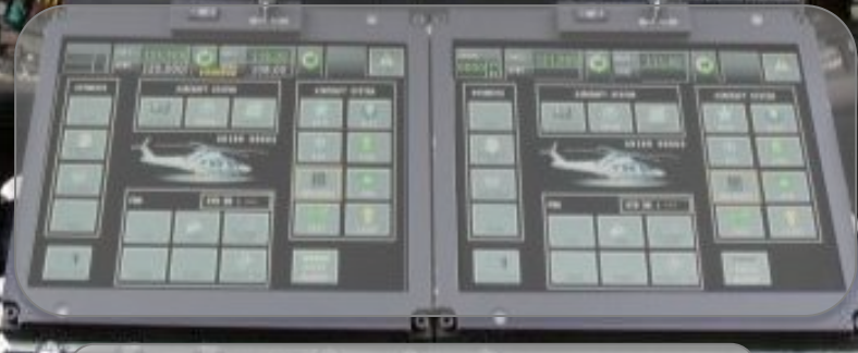
Enhanced Display & Control Units (EDCUs) Touchscreen
