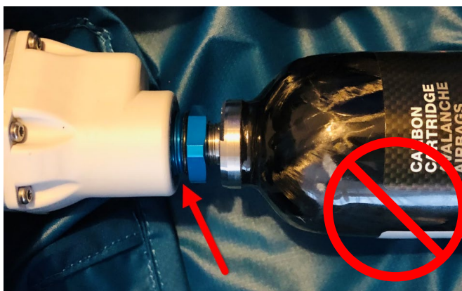
Figure: INCORRECTLY installed cartridge in the mechanism of the airbag inflation system - black rubber seal is still visible.
