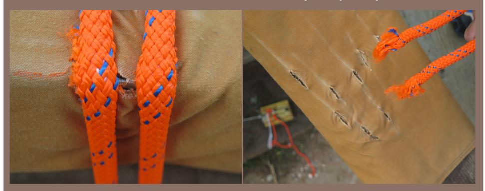
LESS TENSIONED ROPES ARE LESS LIKELY TO BE DAMAGED/ CUT FROM SHARP EDGES
