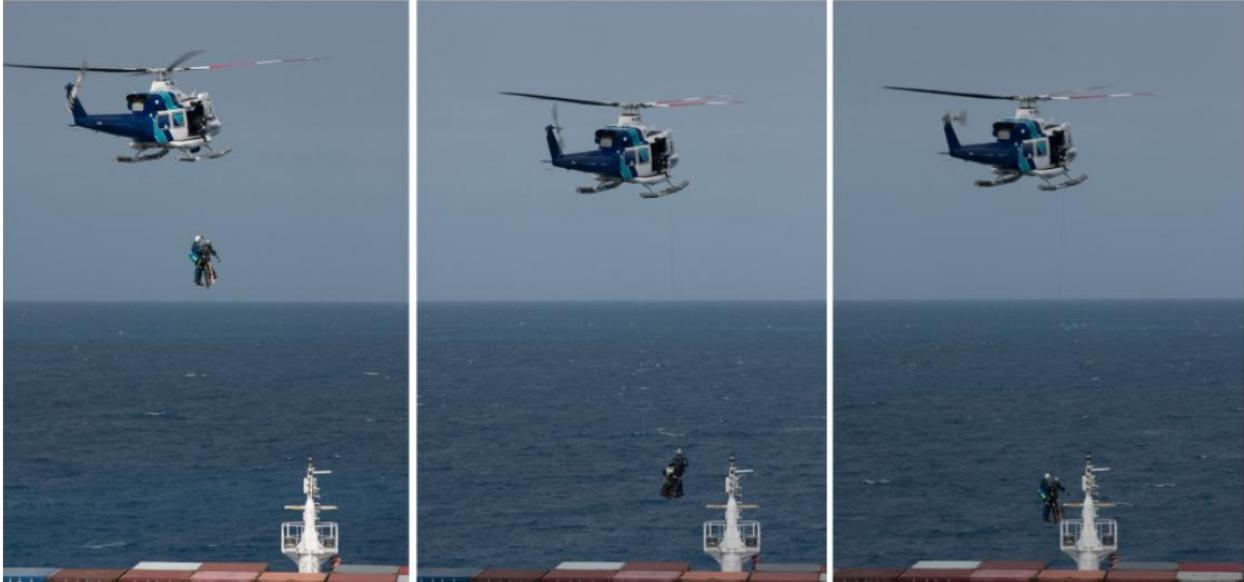
drifting back towards a mast that was located on the forecastle. Despite assistance from the hoist operator to re-establish the hover, the pilot was unable to arrest the helicopter's movement and the hoist cable became fouled while the helicopter continued to drift rearwards. The winch cable separated.
