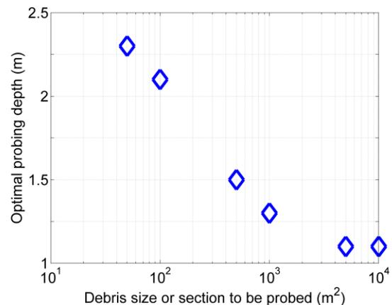
Figure 1: Most survival chance optimized probing depth in the first pass for different sizes of the probed section of the debris.
