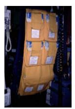
A custom pocket system fastened to the back of the copilots seat provides storage for all the map coverage for the area serviced by this helicopter.
