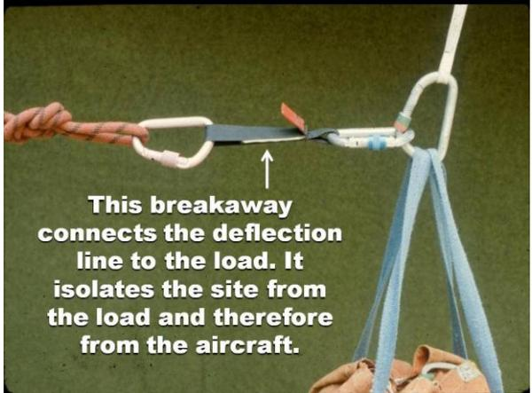
**This breakaway connects the deflection line to the load. It isolates the site from the load and therefore from the aircraft.**
