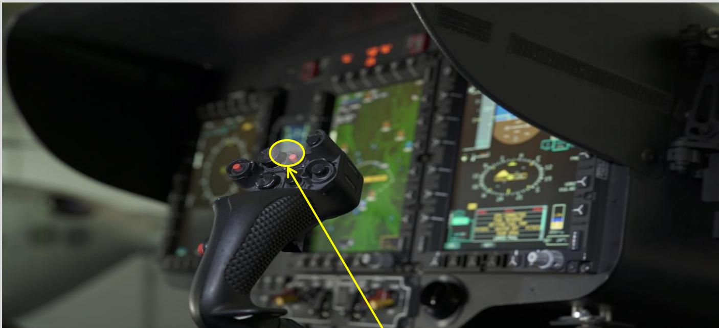
In case of reference attitude lose, one double-click on cyclic stick will stabilize the aircraft to level flight (no turn or climb/descent and steady speed)
