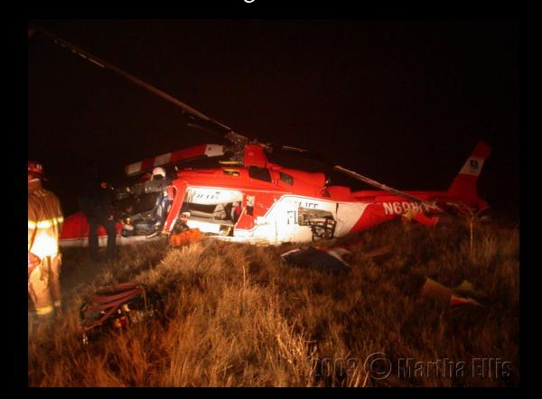
Life Flight 6 was destroyed when it impacted terrain. The pilot and flight paramedic were fatally injured, and the flight nurse was seriously injured.
