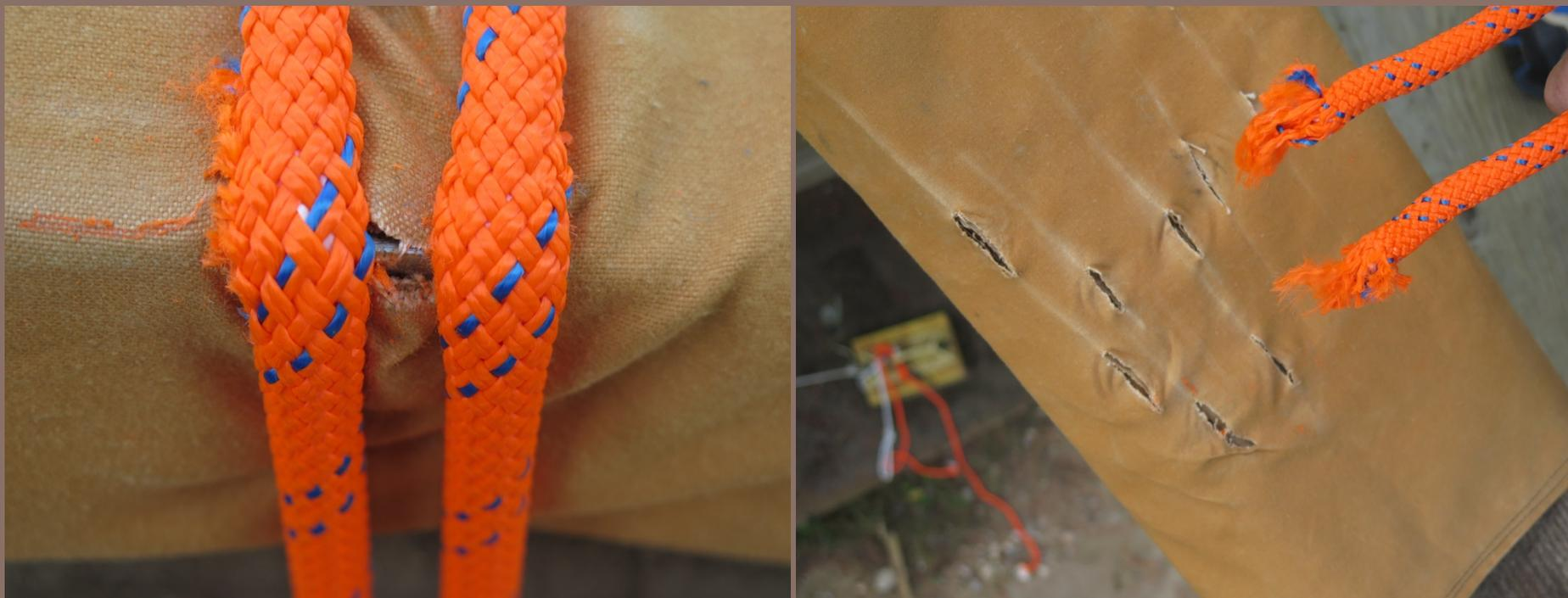
**LESS TENSIONED ROPES ARE LESS LIKELY TO BE DAMAGED/
