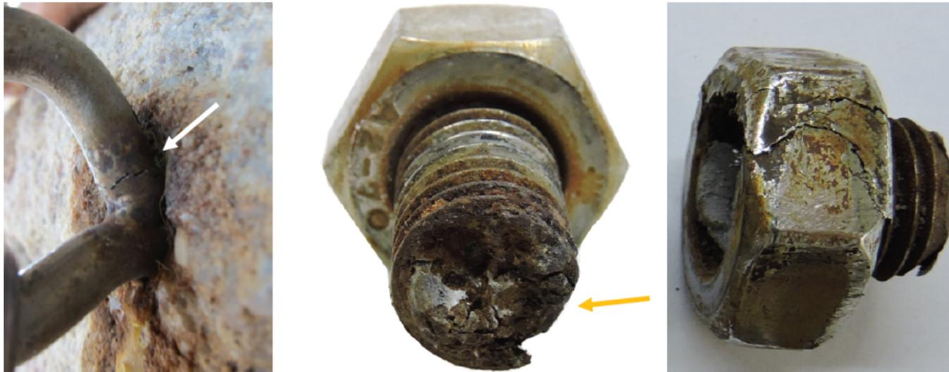
Fig. 14 – Left: Crack on the eye of P-type anchor, initiated from a crevice between anchor and rock; Center: failed TCE bolt with almost completely corroded fracture surface; Right: failed bolt with cracked nut. Arrows show the SCC initiation sites.
