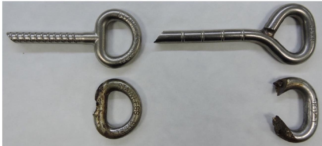
Fig. 16 - Original (top) and failed (bottom) P-type anchors from Taiwan. Left: forged; right: welded.
