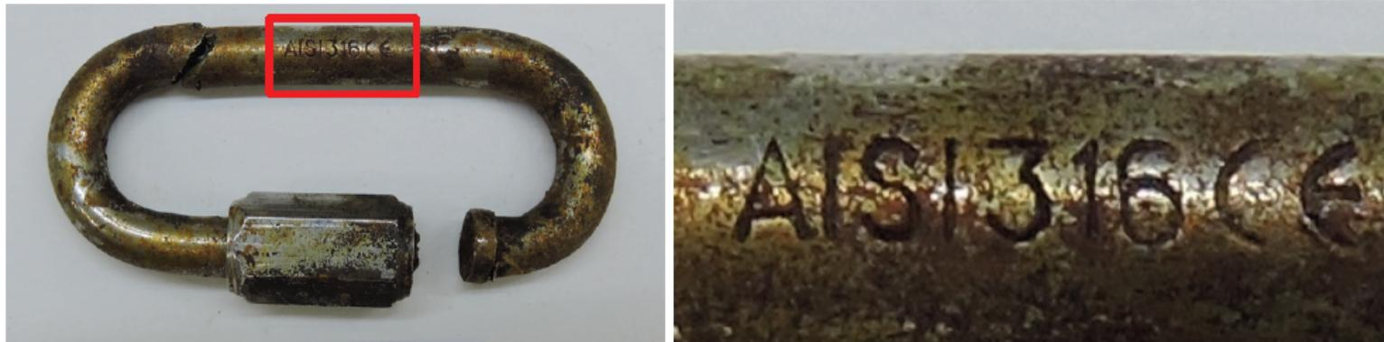
Fig. 15 - Failed quicklink made of low quality SS with false designation (sample P15).
