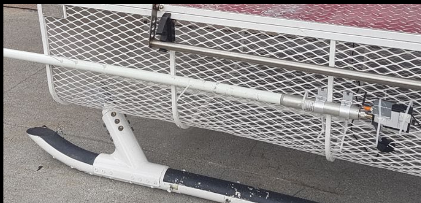
Resero Heli SAR prototype with omnidirectional 8 Db antenna mounted at the helicopter
