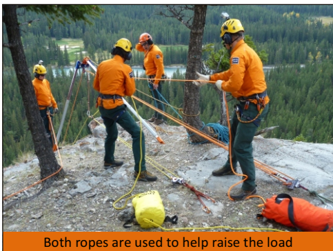
Both ropes are used to help raise the load
