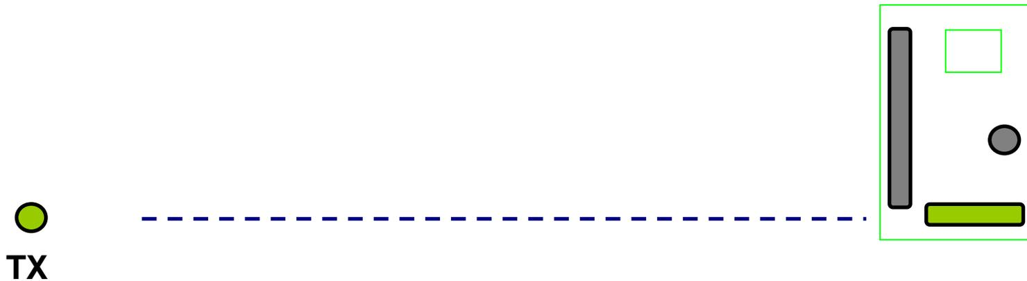
**Test with vertical Transmitter 0Hz, 80Hz and -80Hz deviation!!**
