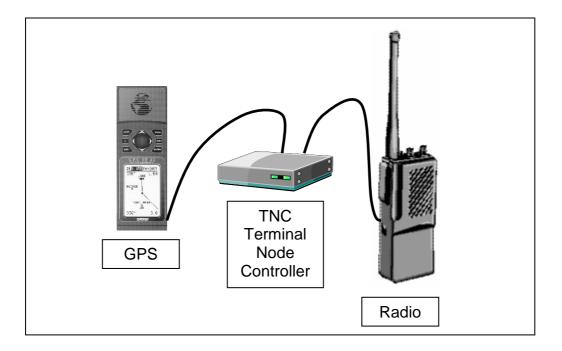
At the control centre, the incoming signal can be decoded by another TNC, and then directed to a serial port on the computer. As each TNC can be programmed separately, each rescue team member can be individually tracked on the map on the computer screen. If required, the progress
