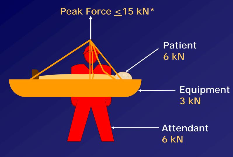
\* Typical peak force is less than 12 kN
